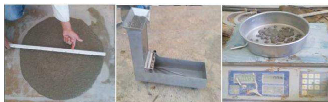
Fig. 3 Qualification test of self-compacting concrete: a-Slump flow, b- L-Box and c-Stability in sieve
